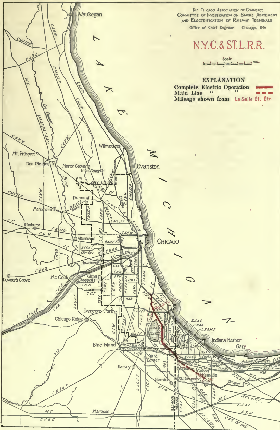
FIG. 571. TRACKAGE TO BE ELECTRIFIED BY THE NEW YORK, CHICAGO & ST. LOUIS RAILROAD
